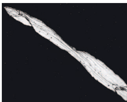
Figure 15. Edge Micrograph of a U6Nb Fragment
